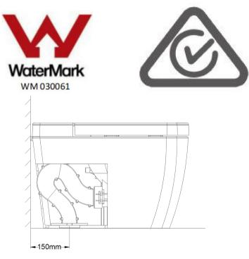
Notice : Rought-in distance should be 150mm if the toilet is against rear wall. Water Pressure:0.15MPa-0.75MPa(dynamic pressure 1.5-static pressure 7.5kg) minimum flowrate is 5L/8s.
